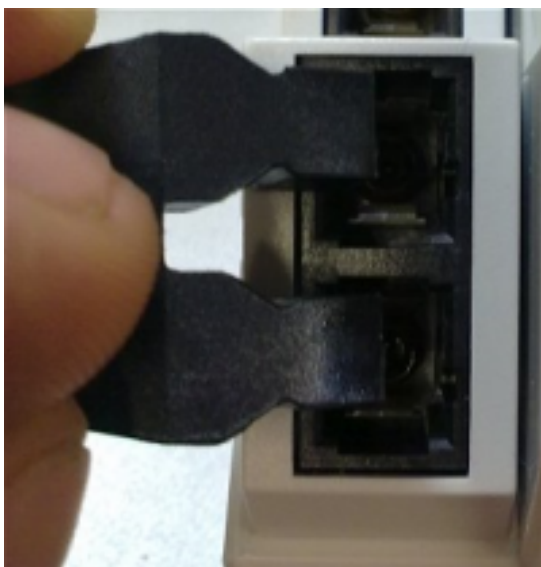
Figure: Blind plugs in unused sockets
