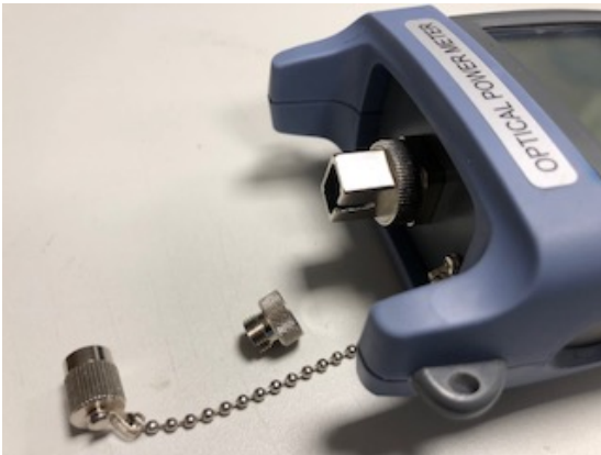
OPM with SC adapter screwed on
