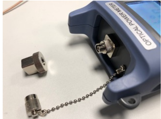
OPM with FC adapter screwed on
