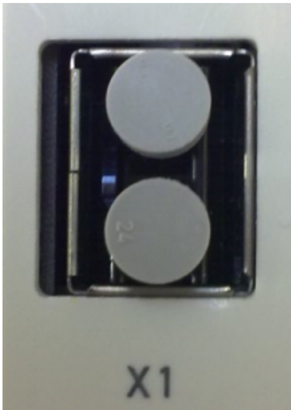
Figure: Blind plugs in unused sockets
