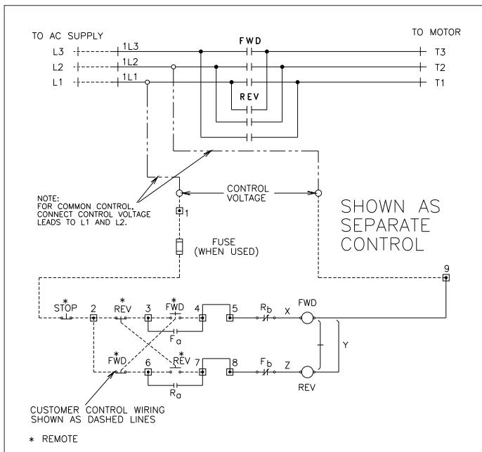
**Figure 7. Reversing Control Circuit**
