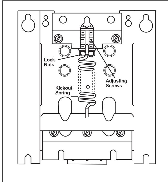
**Figure 8. Kickout Spring**
