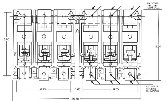
Figure 3. Reversing and Nonreversing Contactor (V211, V201) Dimension Drawing (Dim. in inches)
