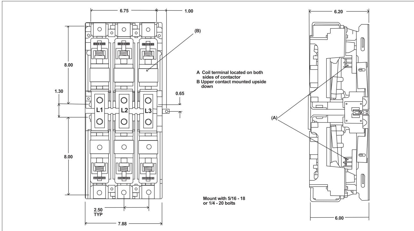
Figure 4. Reversing Controller (V251) Dimension Drawing (Dimensions in inches)
