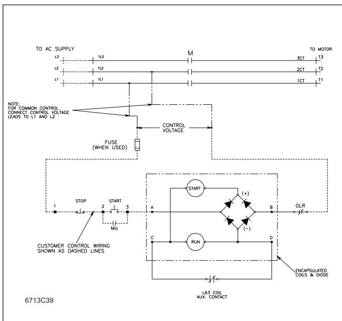
**Figure 6. Connection Diagram, V201**
