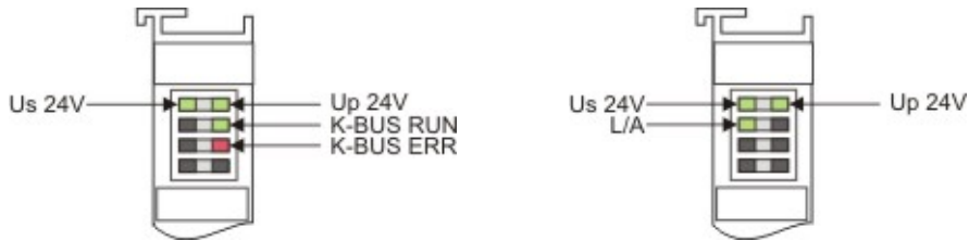
Operation with K-bus terminals
