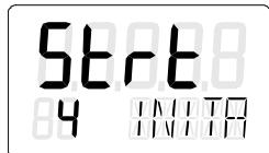
The positioner runs through five initialization steps during the automatic initialization process. The displays for the initialization steps from "RUN 1" to "RUN 5" are located in the lower line of the display. The initialization process depends on the actuator used, and takes up to 15 minutes.
