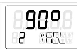
3. Check whether the value displayed in the "2.YAGL" parameter matches the setting of the transmission ratio selector. If required, change the setting of the transmission ratio selector to 33° or 90°.
