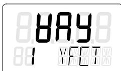
2. Use the
