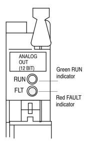
The front panel of the module contains a green RUN and a red FLT (fault) indicator. Possible module fault causes and corrective actions are shown in the table below.
