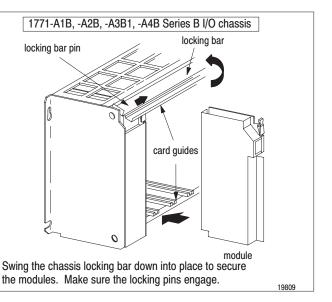
The 1771–OFE modules are a modular component of the 1771 I/O system requiring a properly installed system chassis. Refer to publication 1771–IN075 for detailed information on acceptable chassis and proper installation and grounding requirements. Limit the maximum adjacent slot power dissipation to 10W maximum.
