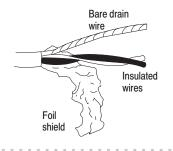
Twist the foil shield and drain wire together to form a single strand.
