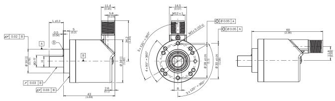
① Measuring point for operating temperature
