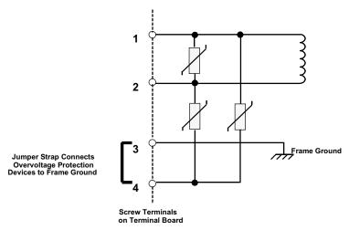
Figure 4-3. Overvoltage Protection Devices and Jumper Strap
