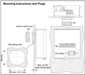
The junction box JB 001 is used to connect a KeTop to a KEMRO PLC. The connection can be realized via the interfaces Ethernet as well as RS-232-C or RS-422-A. The CAN interface S4 is not used.
