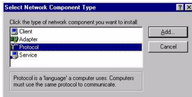
Fig. 5-8: Control Panel / Network / add protocol
