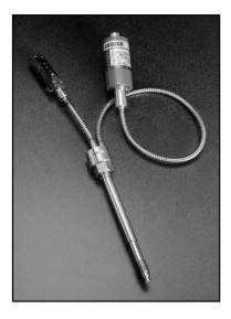
Maximum pressure: 2 x full range or 35,000 psi (whichever is less) Material in contact with pressure media: 15 - 5 PH stainless steel, Armoloy coated Weight: 2.5 lbs. Thermocouple: Type J
