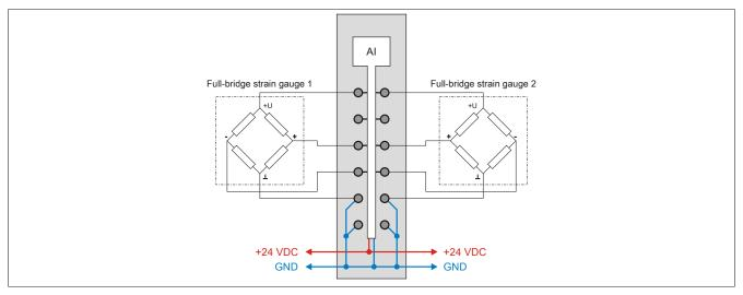
When connecting 3 or more full-bridge strain gauges in parallel, 2 lines must be connected together in an X20 terminal block.
