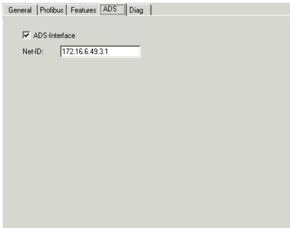
Fig. 124: DP master, ADS tab: Activating the ADS interface and entering the Net ID
