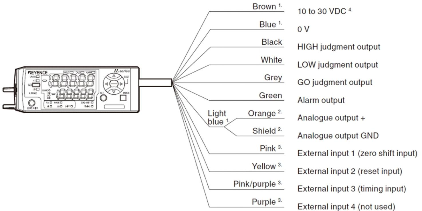
1. The brown, blue, and light blue cables are not provided in a IL-1050/IL-1550 unit (expansion unit).
