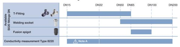
Note A: Only use plastic fitting in analytical version with true union acc. to DIN 8063 (PVC), to DIN 16962 (PP) or to ISO 10931 (PVDF).
